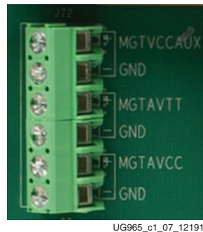
Figure 1-7: GTH Transceiver Power Terminal Block J72
