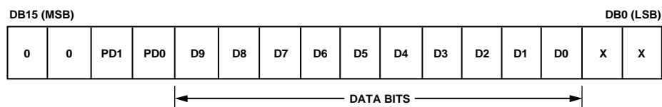
Figure 40. AD5612 Input Register Contents
