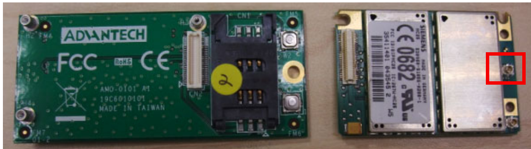
Figure 5.10 AMO-EDGE base board and Siemens module
