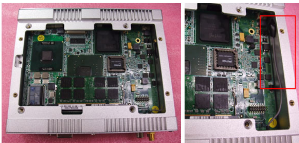
Figure 5.4 GPRS/EDGE SMA cable internally
