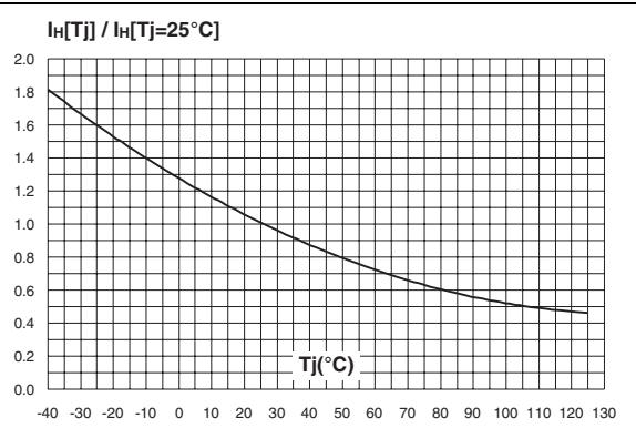
**Figure 6. Relative variation of breakdown voltage versus junction temperature**
