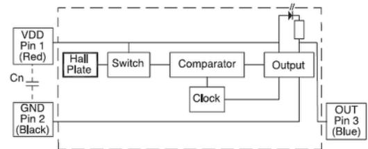
Note: Add capacitor Cn as shown, close for the sensors for transient suppression if required.
