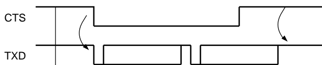
Figure 33-29. Transmitter Behavior when Operating with Hardware Handshaking
