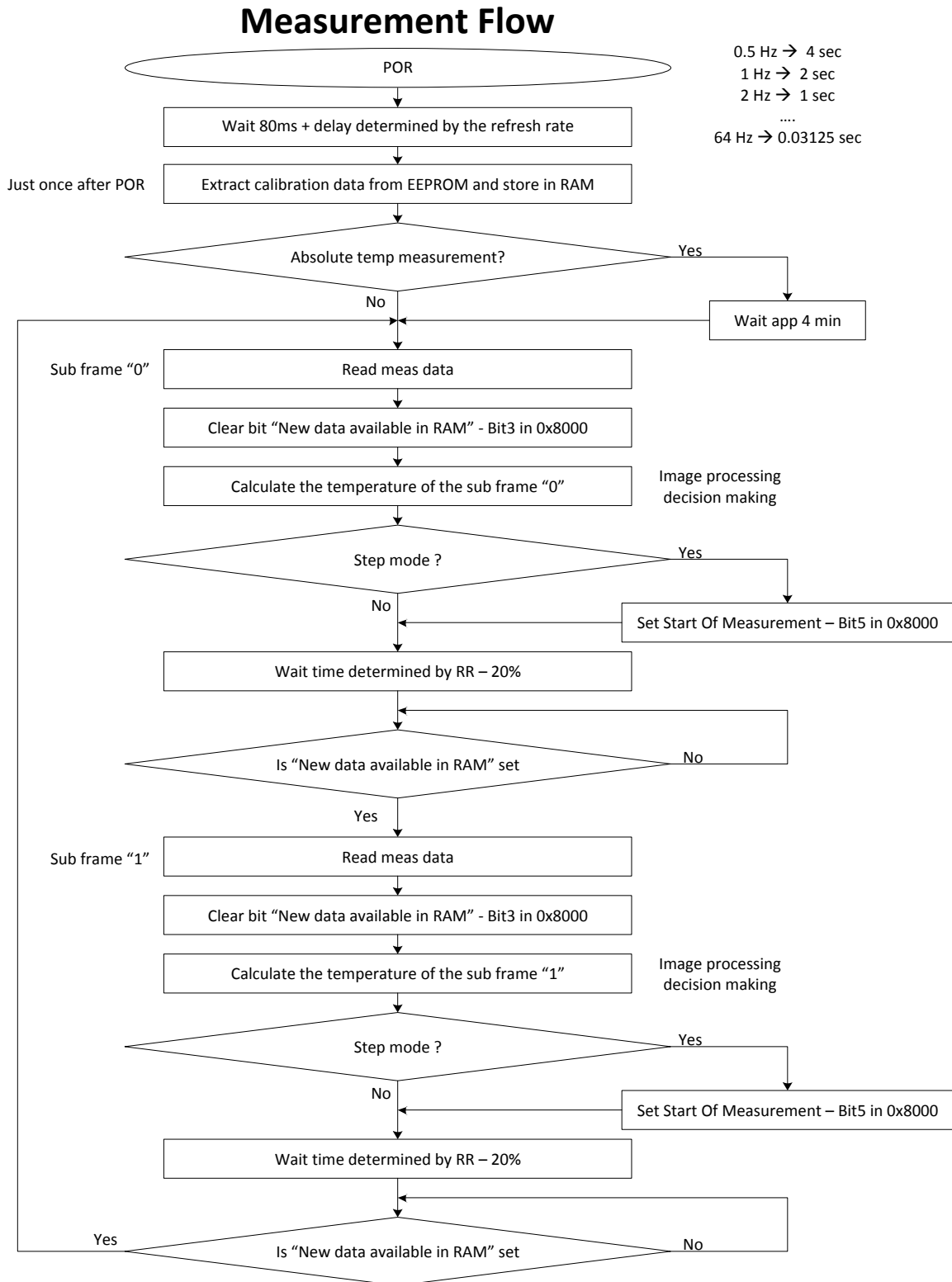
Figure 7 Recommended measurement flow
