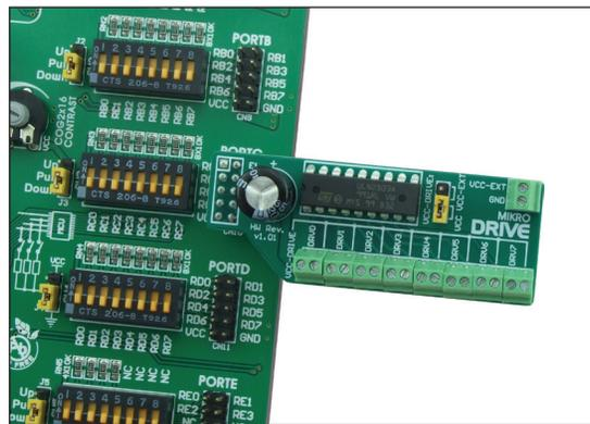
Figure 2: *mikroDRIVE* connected to a development system
