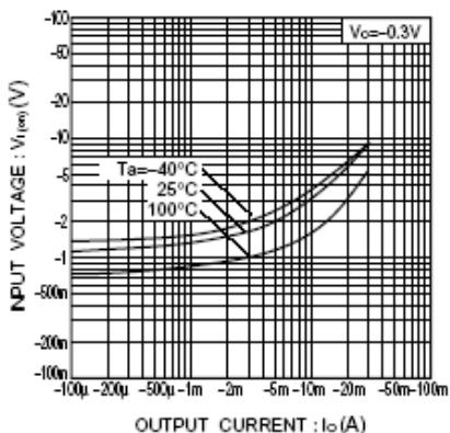
Fig.1 Input voltage vs. output current
