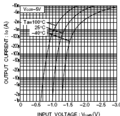
Fig.2 Output current vs. input voltage
