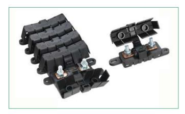
The MEGA®-FLEX fuse holder is used with the MEGA® style bolt-down fuse, which is available up to 500A. This holder offers a flexible cover, which allows cable entry from virtually any direction, large wire size, and ring terminal stack up. Slots on the base allow holder to be mounted with tie wraps. Dovetail features allow you to interlock multiple MEGA®-FLEX fuse holders together for a high power distribution block. Bus bars are avalable for multiple holder applications.
