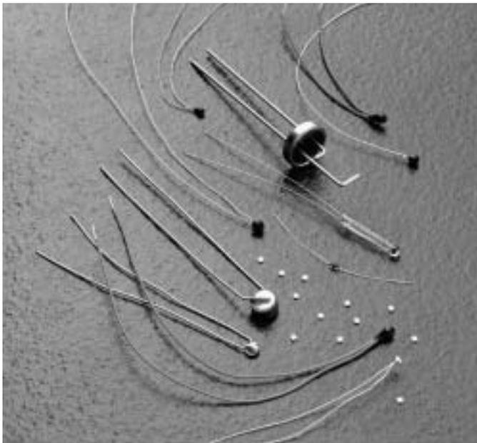
Thermistors change resistance with a change in temperature. They do not amplify, rectify, polarize or generate a signal. The thermistor temperature may be changed by the surrounding temperature or by self-heating the thermistor by passing a current through it.
