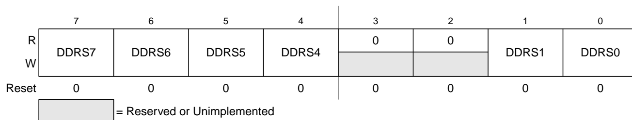
Figure 4-32. Port S Data Direction Register (DDRS)
