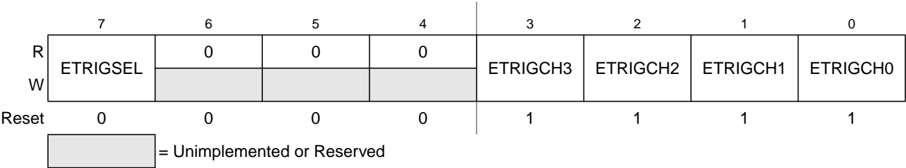
Figure 7-4. ATD Control Register 1 (ATDCTL1)
