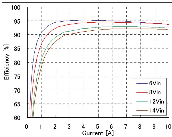
**Fig-2.5V-2:** Efficiency vs. load current and input voltage for  $V_{out}=2.5V$ .
