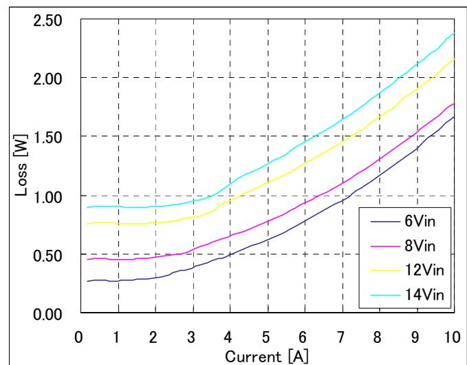
**Fig-3.3V-3:** Power Loss vs. load current and input voltage for  $V_{out}=3.3V$ .
