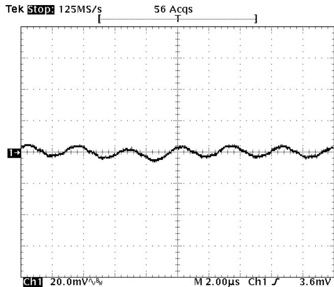
**Fig-1.0V-5:** Output voltage ripple (20mV/div.) for  $V_{\text{out}}=1.0\text{V}$  at full rated load current into a resistive load with external capacitance  $47\mu\text{F}\times 2$  ceramic +  $1\mu\text{F}$  ceramic at  $V_{\text{in}}=12\text{V}$ .
