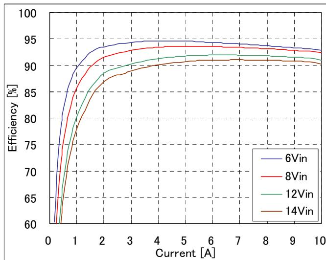
**Fig-2.0V-2:** Efficiency vs. load current and input voltage for  $V_{out}=2.0V$ .
