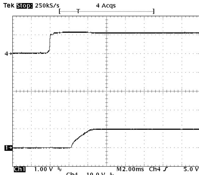
**Fig-1.0V-4:** Turn-on transient for  $V_{\text{out}}=1.0\text{V}$  with application of  $V_{\text{in}}$  at full rated load current (resistive) and  $47\mu\text{F}\times 2$  external capacitance at  $V_{\text{in}}=12\text{V}$ .
