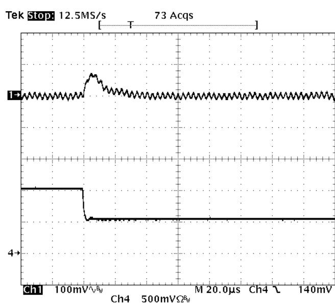
**Fig-2.0V-7:** Output voltage response for  $V_{out}=2.0V$  to negative load current step change from 10A to 5A with slew rate of  $-5A/\mu s$  at  $V_{in}=12V$ .  $C_o=47\mu Fx2$  ceramic.
