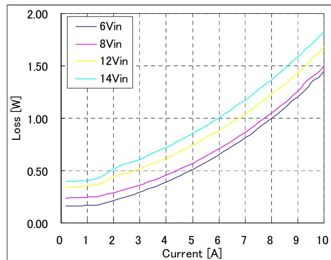
**Fig-1.2V-3:** Power Loss vs. load current and input voltage for  $V_{out}=1.2V$ .
