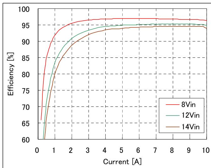
**Fig-5.0V-2:** Efficiency vs. load current and input voltage for  $V_{out}=5.0V$ .
