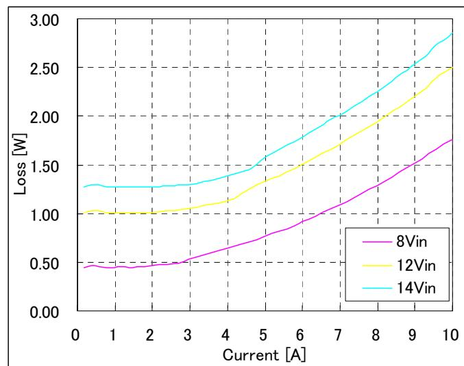
**Fig-5.0V-3:** Power Loss vs. load current and input voltage for  $V_{out}=5.0V$ .
