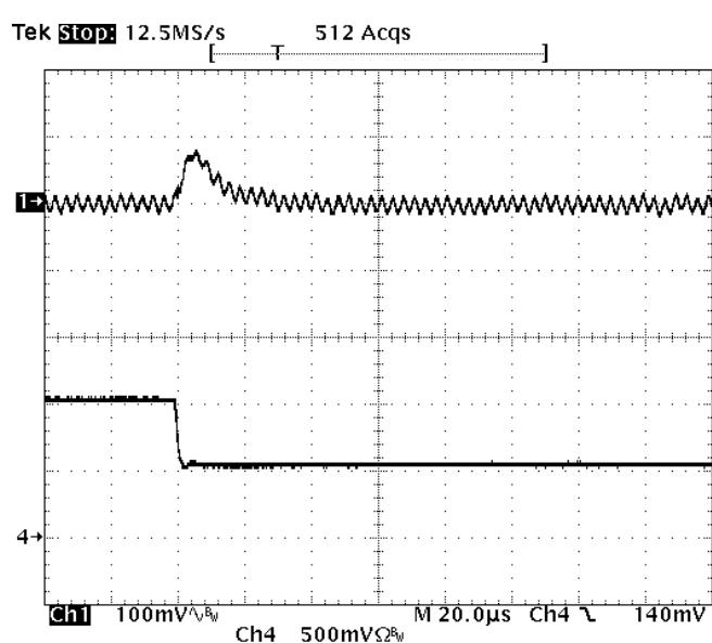
**Fig-2.5V-7:** Output voltage response for  $V_{out}=2.5V$  to negative load current step change from 10A to 5A with slew rate of  $-5A/\mu s$  at  $V_{in}=12V$ .  $C_o=47\mu Fx2$  ceramic.
