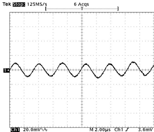
**Fig-2.5V-5:** Output voltage ripple (20mV/div.) for  $V_{out}=2.5V$  at full rated load current into a resistive load with external capacitance  $47\mu Fx2$  ceramic +  $1\mu F$  ceramic at  $V_{in}=12V$ .
