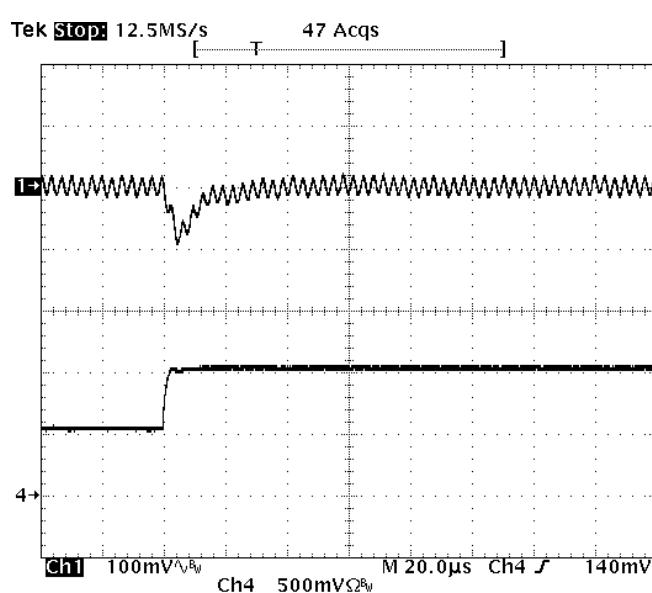
**Fig-3.3V-6:** Output voltage response for  $V_{out}=3.3V$  to positive load current step-change from 5A to 10A with slew rate of  $5A/\mu s$  at  $V_{in}=12V$ .  $C_o=47\mu Fx2$  ceramic.
