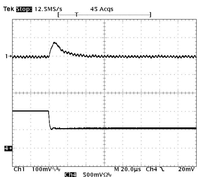
**Fig-1.0V-7:** Output voltage response for  $V_{\text{out}}=1.0\text{V}$  to negative load current step change from 10A to 5A with slew rate of  $-5\text{A}/\mu\text{s}$  at  $V_{\text{in}}=12\text{V}$ .  $C_{\text{o}}=47\mu\text{F}\times 2$  ceramic.
