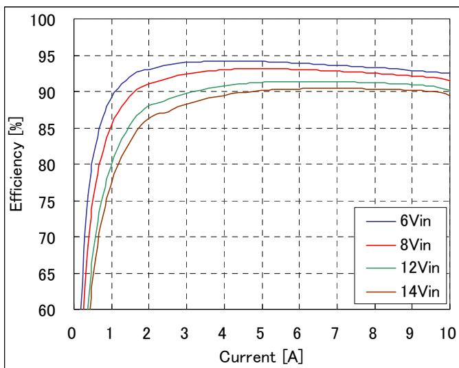
**Fig-1.8V-2:** Efficiency vs. load current and input voltage for  $V_{out}=1.8V$ .
