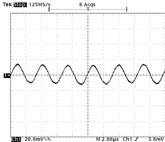
**Fig-3.3V-5:** Output voltage ripple (20mV/div.) for  $V_{out}=3.3V$  at full rated load current into a resistive load with external capacitance  $47\mu Fx2$  ceramic +  $1\mu F$  ceramic at  $V_{in}=12V$ .
