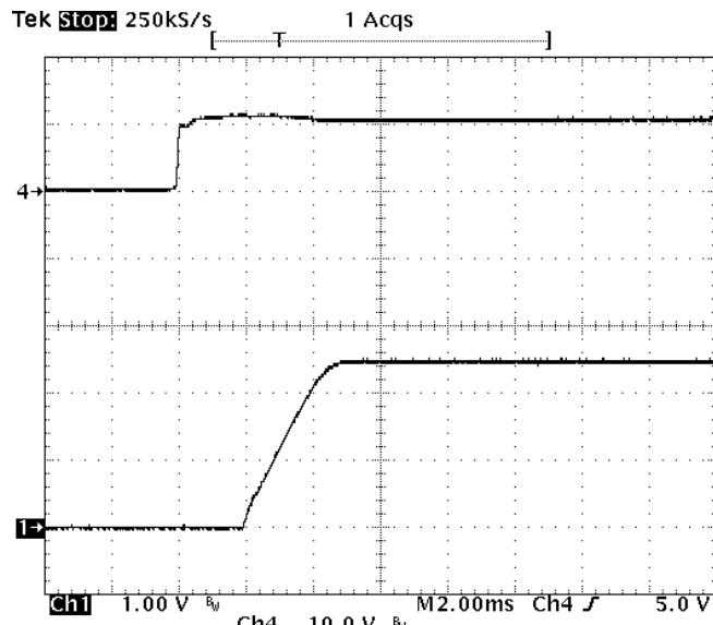
**Fig-2.5V-4:** Turn-on transient for  $V_{out}=2.5V$  with application of  $V_{in}$  at full rated load current (resistive) and  $47\mu Fx2$  external capacitance at  $V_{in}=12V$ .
