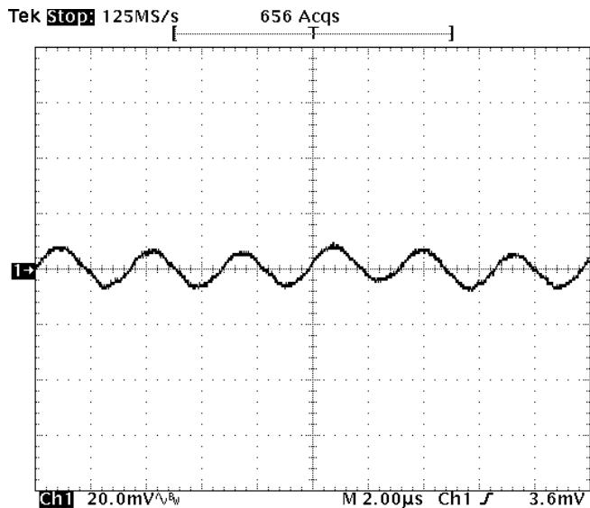
**Fig-1.8V-5:** Output voltage ripple (20mV/div.) for  $V_{out}=1.8V$  at full rated load current into a resistive load with external capacitance  $47\mu Fx2$  ceramic +  $1\mu F$  ceramic at  $V_{in}=12V$ .
