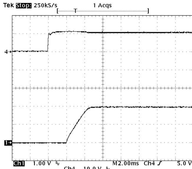
**Fig-2.0V-4:** Turn-on transient for  $V_{out}=2.0V$  with application of  $V_{in}$  at full rated load current (resistive) and  $47\mu Fx2$  external capacitance at  $V_{in}=12V$ .
