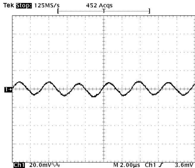
**Fig-2.0V-5:** Output voltage ripple (20mV/div.) for  $V_{out}=2.0V$  at full rated load current into a resistive load with external capacitance  $47\mu Fx2$  ceramic +  $1\mu F$  ceramic at  $V_{in}=12V$ .
