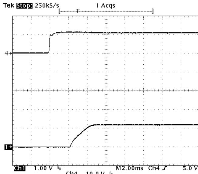
**Fig-1.2V-4:** Turn-on transient for  $V_{out}=1.2V$  with application of  $V_{in}$  at full rated load current (resistive) and  $47\mu Fx2$  external capacitance at  $V_{in}=12V$ .
