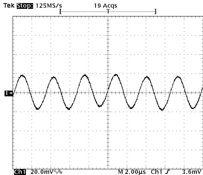
**Fig-5.0V-5:** Output voltage ripple (20mV/div.) for  $V_{out}=5.0V$  at full rated load current into a resistive load with external capacitance  $47\mu Fx2$  ceramic +  $1\mu F$  ceramic at  $V_{in}=12V$ .
