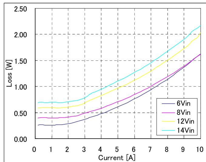
**Fig-2.5V-3:** Power Loss vs. load current and input voltage for  $V_{out}=2.5V$ .
