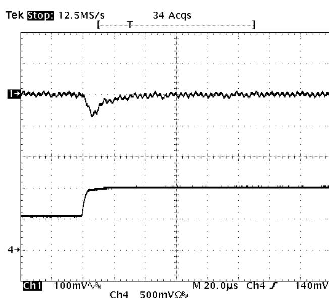
**Fig-1.2V-6:** Output voltage response for  $V_{out}=1.2V$  to positive load current step change from  $5A$  to  $10A$  with slew rate of  $5A/\mu s$  at  $V_{in}=12V$ .  $C_o=47\mu Fx2$  ceramic.
