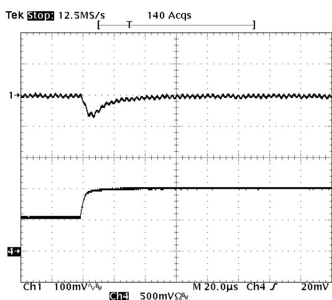
**Fig-1.0V-6:** Output voltage response for  $V_{\text{out}}=1.0\text{V}$  to positive load current step change from 5A to 10A with slew rate of  $5\text{A}/\mu\text{s}$  at  $V_{\text{in}}=12\text{V}$ .  $C_{\text{o}}=47\mu\text{F}\times 2$  ceramic.
