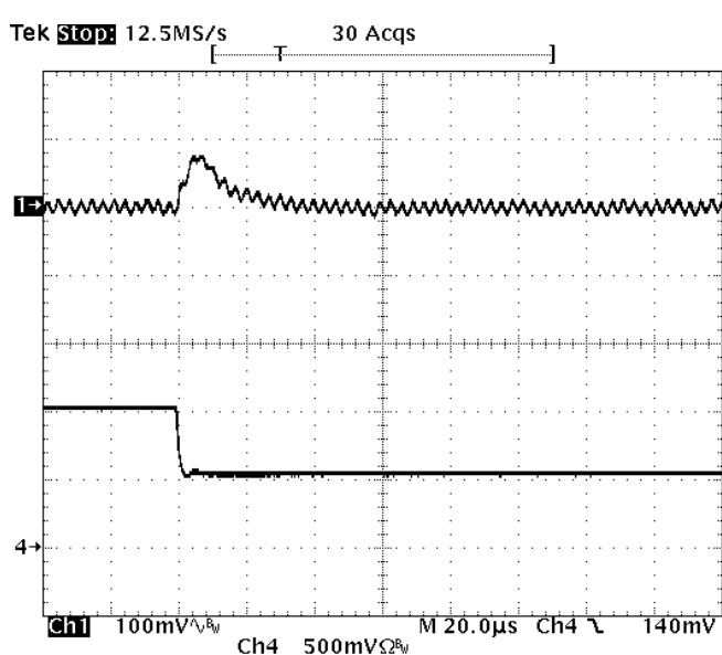
**Fig-1.8V-7:** Output voltage response for  $V_{out}=1.8V$  to negative load current step change from 10A to 5A with slew rate of  $-5A/\mu s$  at  $V_{in}=12V$ .  $C_o=47\mu Fx2$  ceramic.
