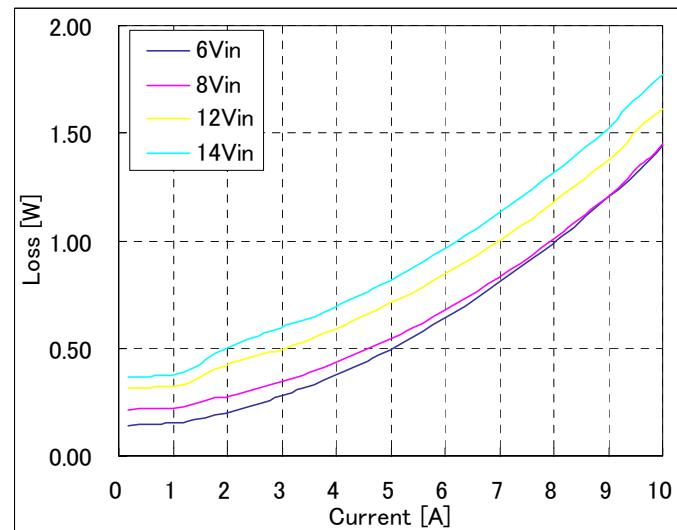
**Fig-1.0V-3:** Power Loss vs. load current and input voltage for  $V_{out}=1.0V$ .
