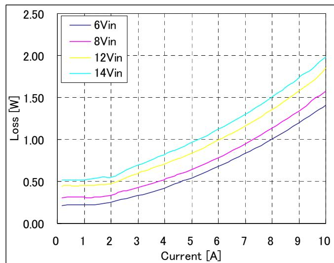
**Fig-1.8V-3:** Power Loss vs. load current and input voltage for  $V_{out}=1.8V$ .
