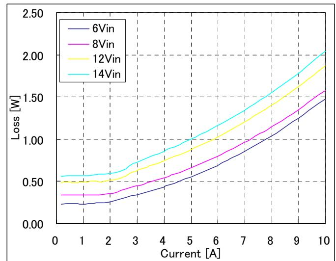
**Fig-2.0V-3:** Power Loss vs. load current and input voltage for  $V_{out}=2.0V$ .
