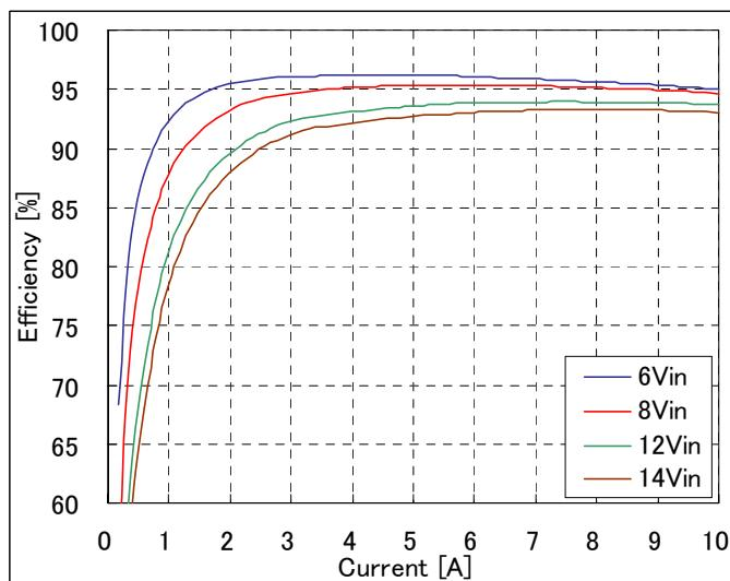
**Fig-3.3V-2:** Efficiency vs. load current and input voltage for  $V_{out}=3.3V$ .
