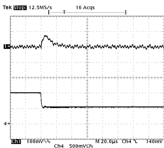
**Fig-1.5V-7:** Output voltage response for  $V_{out}=1.5V$  to negative load current step change from  $10A$  to  $5A$  with slew rate of  $-5A/\mu s$  at  $V_{in}=12V$ .  $C_o=47\mu Fx2$  ceramic.
