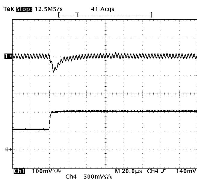
**Fig-2.5V-6:** Output voltage response for  $V_{out}=2.5V$  to positive load current step change from 5A to 10A with slew rate of  $5A/\mu s$  at  $V_{in}=12V$ .  $C_o=47\mu Fx2$  ceramic.
