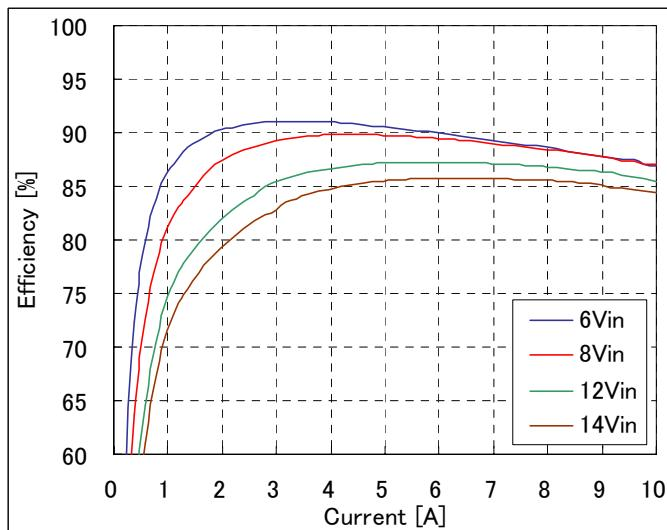
**Fig-1.0V-2:** Efficiency vs. load current and input voltage for  $V_{out}=1.0V$ .
