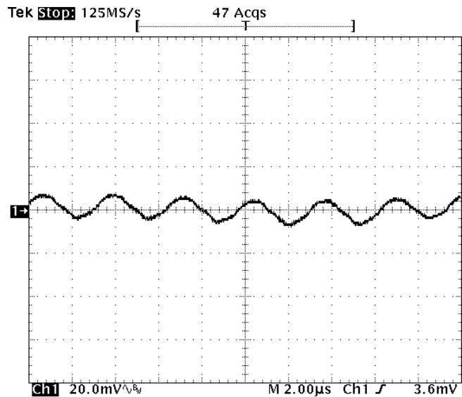
**Fig-1.5V-5:** Output voltage ripple (20mV/div.) for  $V_{out}=1.5V$  at full rated load current into a resistive load with external capacitance  $47\mu Fx2$  ceramic +  $1\mu F$  ceramic at  $V_{in}=12V$ .
