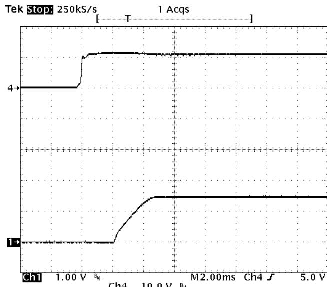
**Fig-1.5V-4:** Turn-on transient for  $V_{out}=1.5V$  with application of  $V_{in}$  at full rated load current (resistive) and  $47\mu Fx2$  external capacitance at  $V_{in}=12V$ .
