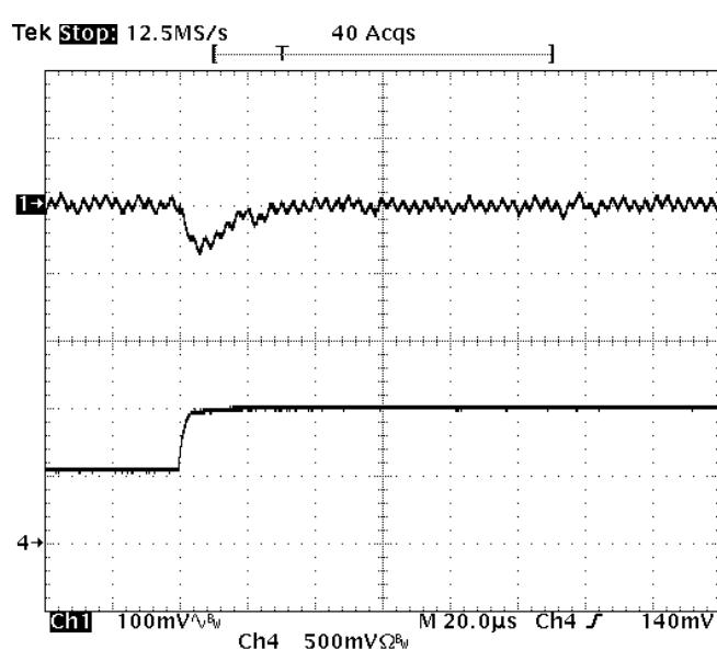
**Fig-1.5V-6:** Output voltage response for  $V_{out}=1.5V$  to positive load current step change from  $5A$  to  $10A$  with slew rate of  $5A/\mu s$  at  $V_{in}=12V$ .  $C_o=47\mu Fx2$  ceramic.
