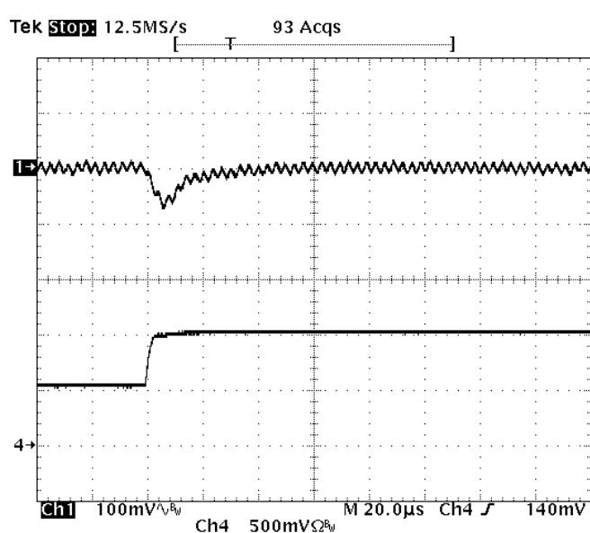
**Fig-1.8V-6:** Output voltage response for  $V_{out}=1.8V$  to positive load current step change from 5A to 10A with slew rate of  $5A/\mu s$  at  $V_{in}=12V$ .  $C_o=47\mu Fx2$  ceramic.
