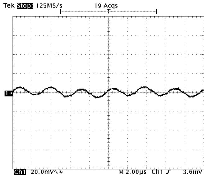
**Fig-1.2V-5:** Output voltage ripple (20mV/div.) for  $V_{out}=1.2V$  at full rated load current into a resistive load with external capacitance  $47\mu Fx2$  ceramic +  $1\mu F$  ceramic at  $V_{in}=12V$ .
