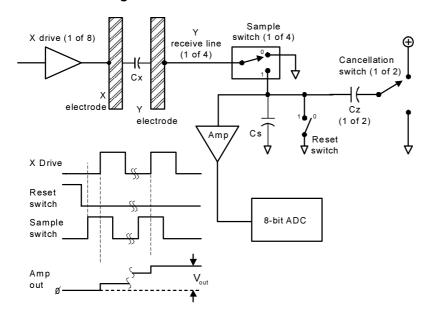
subtract charge from Cs to create a negative-going offset, bringing the signal back to a usable level. This action occurs during the course of the burst and is not illustrated in the timing diagram of Figure 1-4. This mechanism has the benefit of allowing high levels of Cx while remaining highly sensitive to small changes in charge coupling due to touch; the circuit permits the designer to create very large, highly interdigitated touch keys that are very sensitive.
