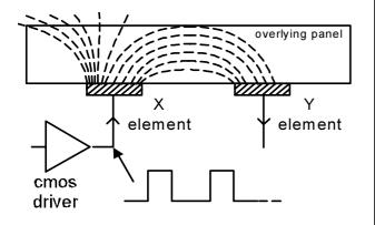
The 60320 uses burst-mode charge transfer methods pioneered and patented by Quantum, including charge cancellation methods which allow for a wide range of key sizes and shapes to be mixed together in a single keypanel. These features permit the construction of entirely new classes of keypanels never before contemplated, such as touch-sliders, back-illuminated keys, and arbitrary shape keypanels, all at very low cost.
