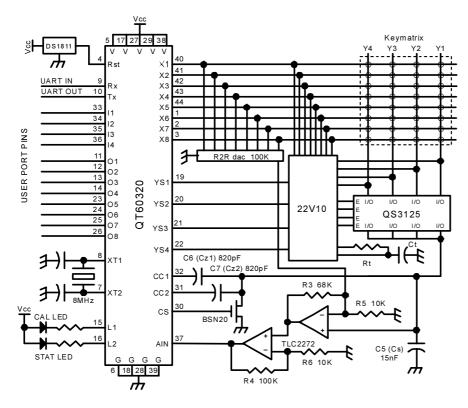
on Cs; each Cz will cancel charge in a discrete step as required.
