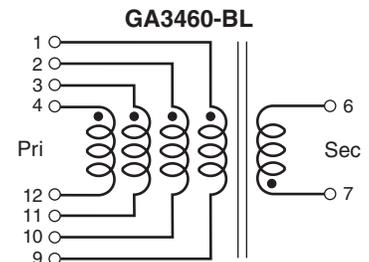
Primary windings to be connected in parallel on PC board.
