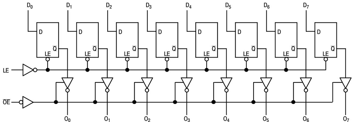
NOTE: That this diagram is provided only for the understanding of logic operations and should not be used to estimate propagation delays.
