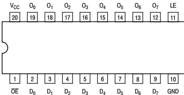
Figure 1. Pinout 20-Lead Packages Conductors (Top View)
