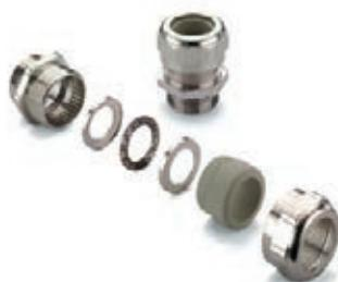
Brass cable gland for shielding against interference frequencies with a screening attenuation of up to 100 dB. Contact with cable shield by means of spring washer.
