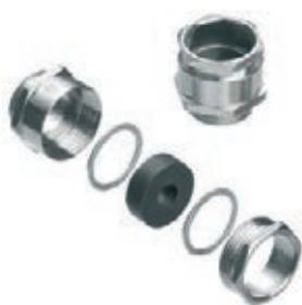
Brass cable gland with incision seal for standard industrial applications. The seal insert which is used contains several removable or separable inlets. This enables cables with a diameter of 4 mm to 41 mm to be connected.
