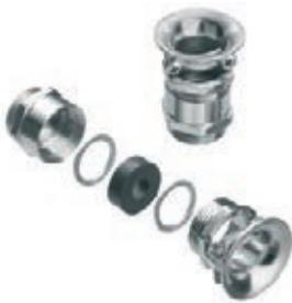
Industrial brass cable glands with strain-relief and trumpet-shaped anti-bend mechanism for connecting non-stationary cables and lines. The seal insert which is used contains several removable or separable inlets.
