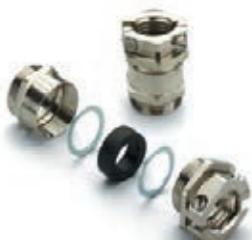
Brass cable glands with external, centrally positioned strain relief provided by clamping jaws. The seal insert which is used contains several removable or separable inlets.
