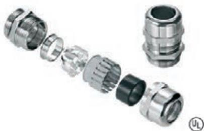
Brass cable gland for shielding against interference frequencies with a shield attenuation of up to 90 dB. Conical metal cage ensures multiple contacts with the cable shielding. On installation, the cable gland does not have to be divided into its individual parts, enabling particularly simple installation.
