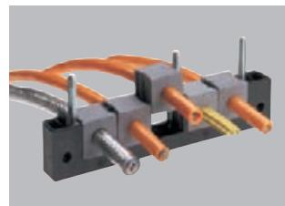
3. Assemble the two halves of the cable entry frame using the M5x50 Allen screws supplied. This achieves integral strain relief in accordance with VDE 0619 (VDE = German Association for Electrical, Electronic and Information Technologies).
