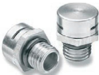
The DAE pressure-compensation element provides good ventilation for the enclosure and prevents moisture build-up. At the same time it maintains the high IP 69k protection level. The membrane repels water and oil.
