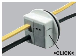
4. Place the seal, which is also supplied, over the thread. Then fit the cable gland into the hole and, if necessary, secure it with a locknut.
