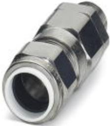
Cable gland, Cable gland material: Nickel-plated brass, Application: Ex, External cable diameter 54.6 mm ... 65.9 mm, Shielding: Yes, Connecting thread: M63, Color: silver
