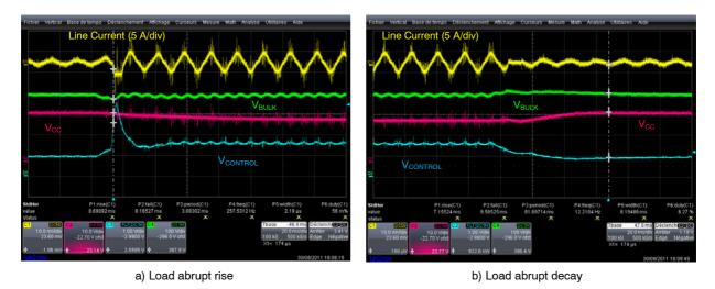
Figure 15. Bulk Voltage Variations when the Load Changes from 100 to 400 mA (2 A/μs slope)
