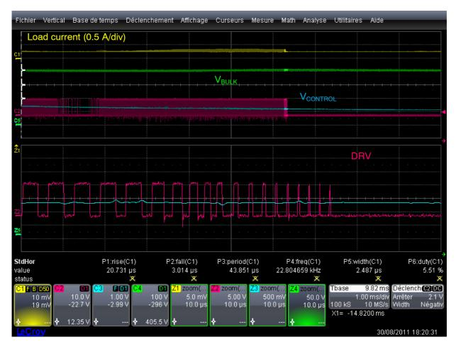
Figure 16. Soft Over-Voltage Protection
