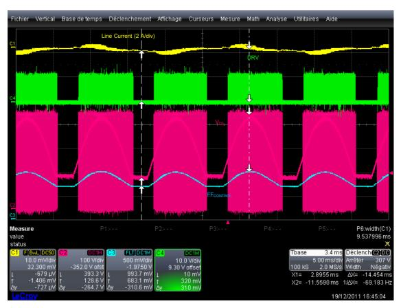
Figure 9. The Circuit Skips Cycle Near the Line Zero Crossing (265 V, 20% Load)
