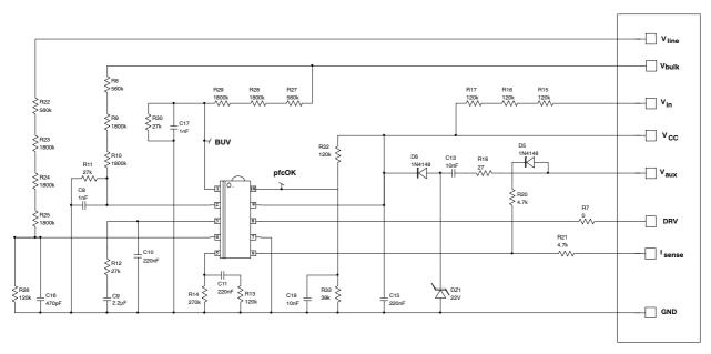
Figure 3. Application Schematic - Control Section
