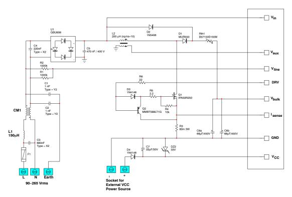
Figure 2. Application Schematic - Power Section
