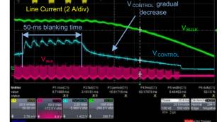
b) Start of operation when V<sub>in,rms</sub> exceeds (V<sub>in,rms</sub>)<sub>BOH</sub> (NCP1612A)
