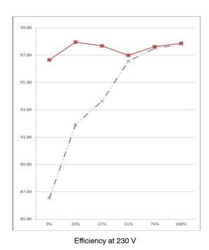
Figure 8. Efficiency versus Load of the Evaluation Board (red solid line), of the Evaluation Board Operated in Full CrM (purple dotted line). In both Cases, the NTC is Shorted.
