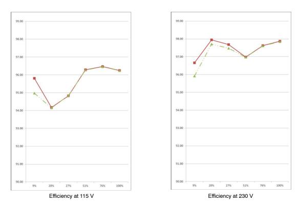
Figure 10. Efficiency versus Load of the Evaluation Board (red solid line) and of the Evaluation Board where Skip Mode is Disabled (green dotted line). In both Cases, the NTC is Shorted.
