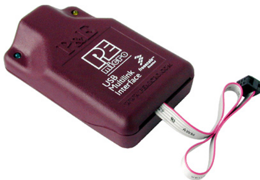
Figure 2. P&E's USB BDM Multilink
