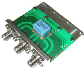
Relay soldered on Test Fixture (2)
