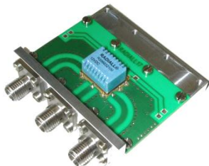
Relay soldered on Test Fixture (2)
