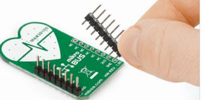
Turn the board upside down so that the bottom side is facing you upwards. Place shorter pins of the header into the appropriate soldering pads.
