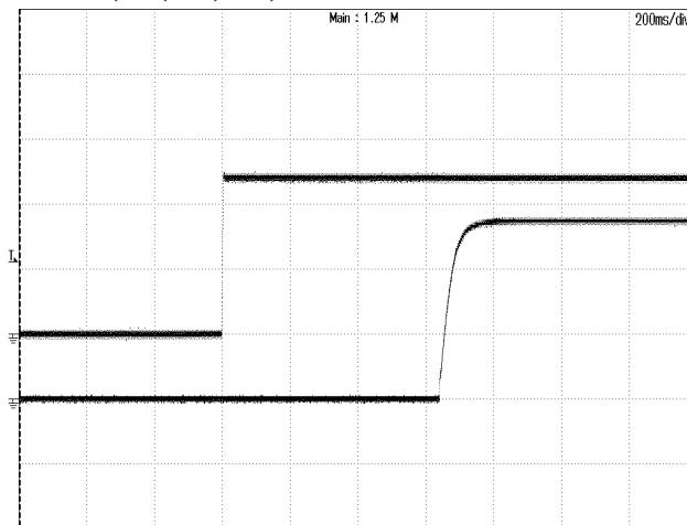
**Figure 4:** Vout start up with Vin on at 48Vin,22A lout,
