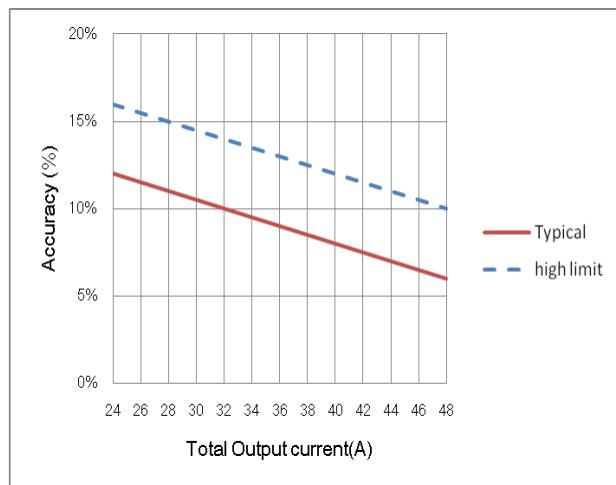
**Figure 10:** Current share accuracy vs. Total output current
