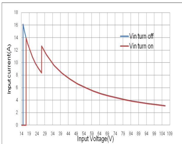
**Figure 7:** Input current vs. Input voltage
