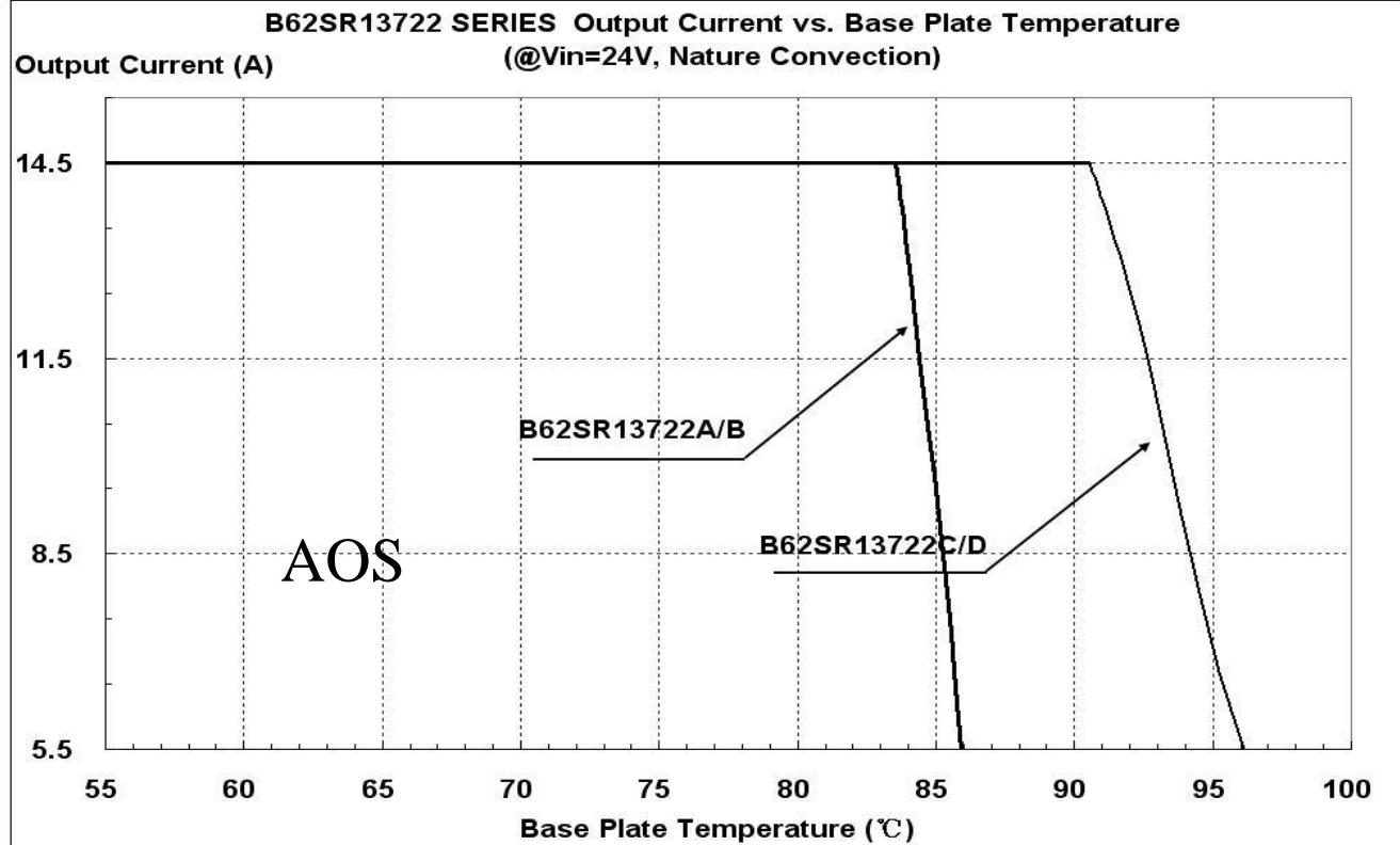
Figure 23: Output Current vs. Base Table temperature @ Vin=24V
