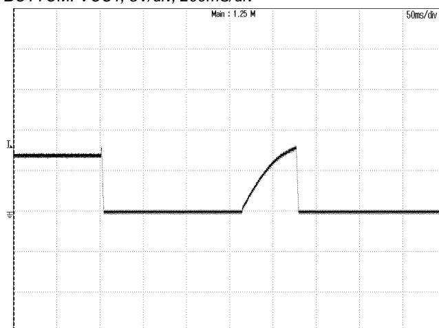
**Figure 6:** Output over voltage protection at 48Vin, 11A lout
