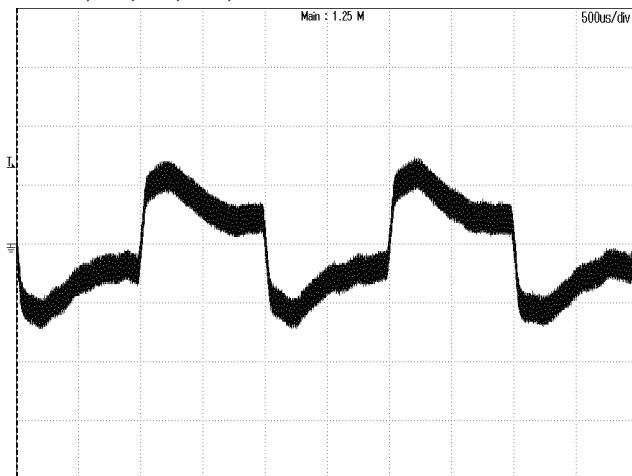
**Figure 3:** Dynamic response to load step 11A~16.5A with 0.1A/uS slew rate at 48Vin
