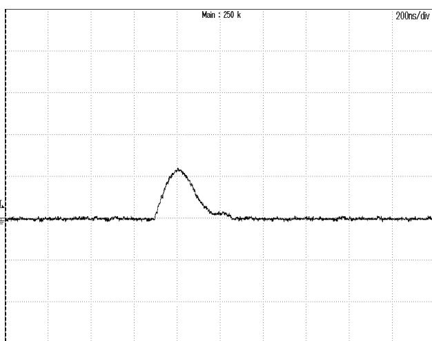
**Figure 11:** Inrush current @ Vin=48V
