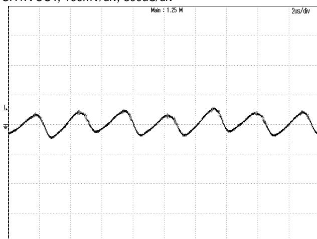
**Figure 5:** Output ripple & noise at 48Vin, 22A lout
