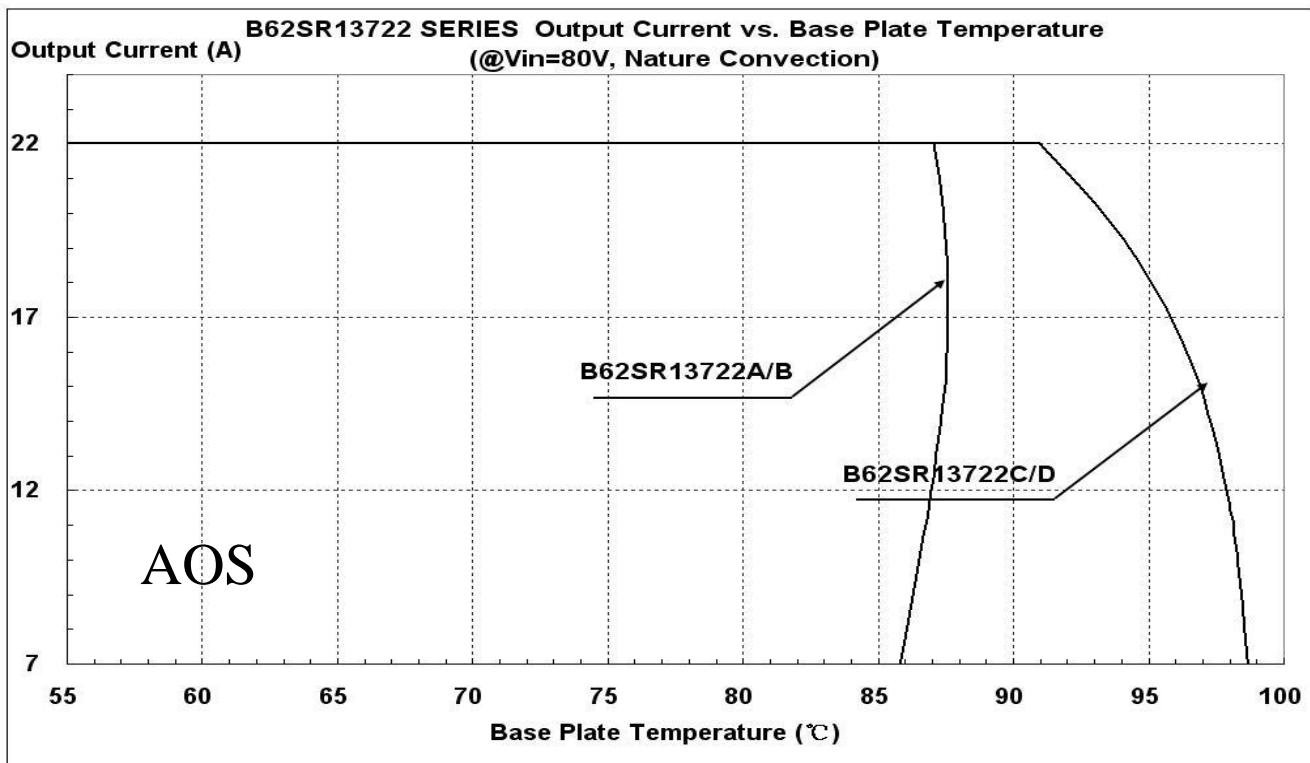
Figure 27: Output Current vs. Base Table temperature @ Vin=80V
