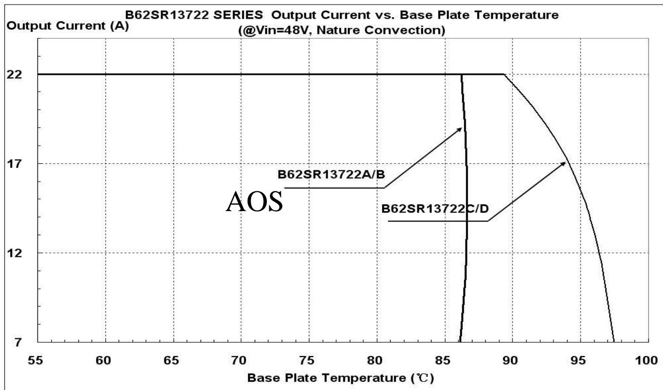
Figure 25: Output Current vs. Base Table temperature @ Vin=48V
