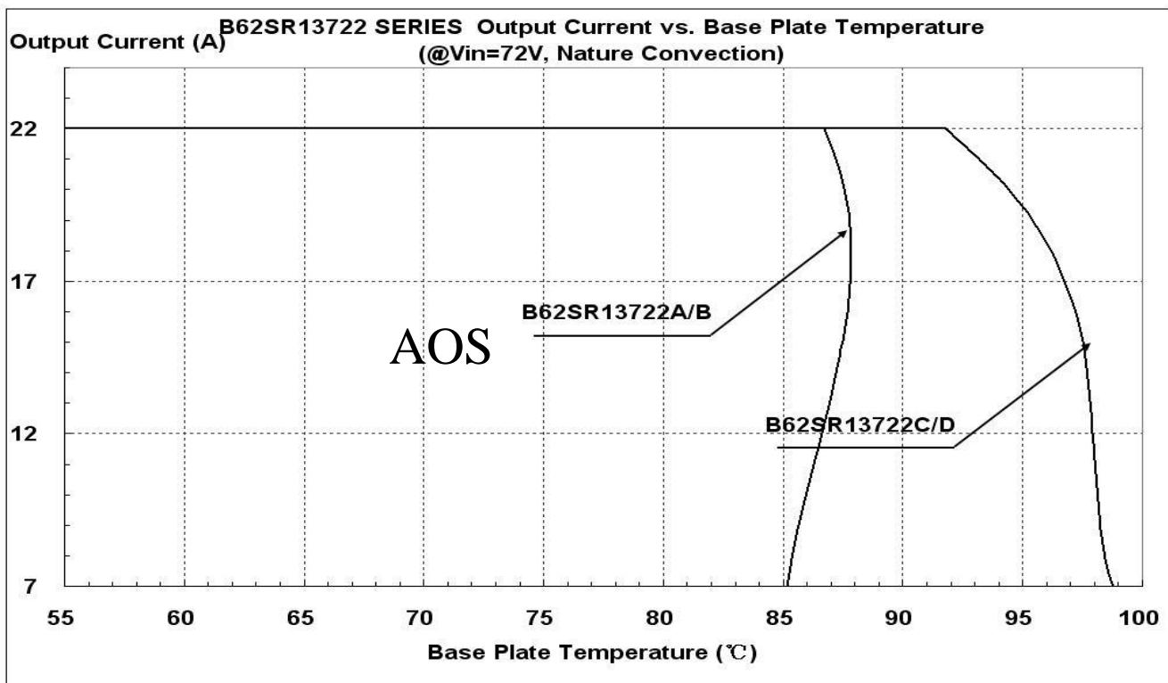
Figure 26: Output Current vs. Base Table temperature @ Vin=72V
