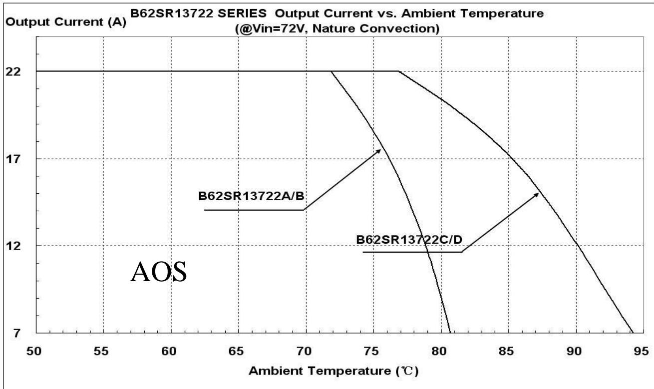
Figure 20: Output Current vs. Ambient temperature @ Vin=72V
