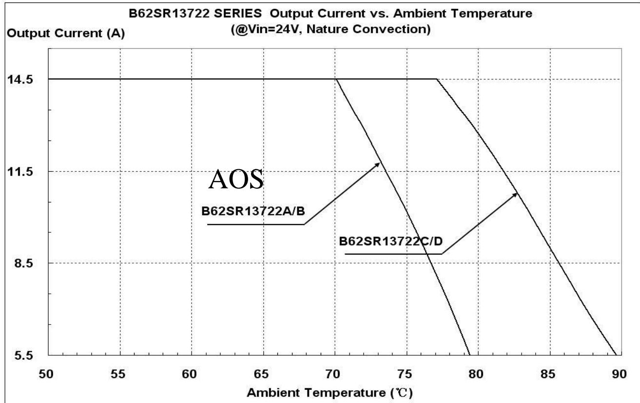
*Figure 17: Output Current vs. Ambient temperature @ Vin=24V*
