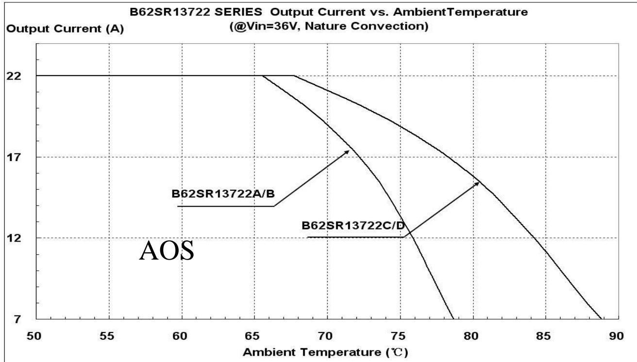
Figure 18: Output Current vs. Ambient temperature @ Vin=36V
