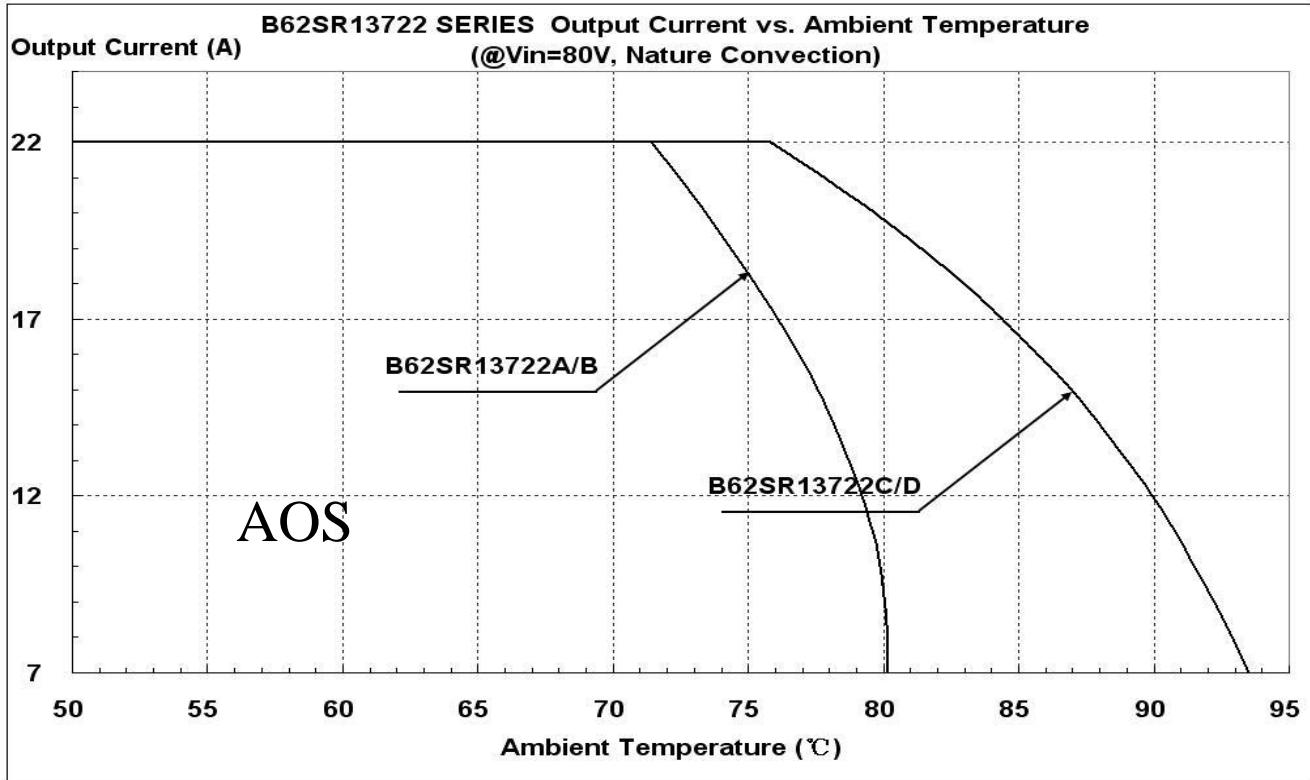
Figure 21: Output Current vs. Ambient temperature @ Vin=80V
