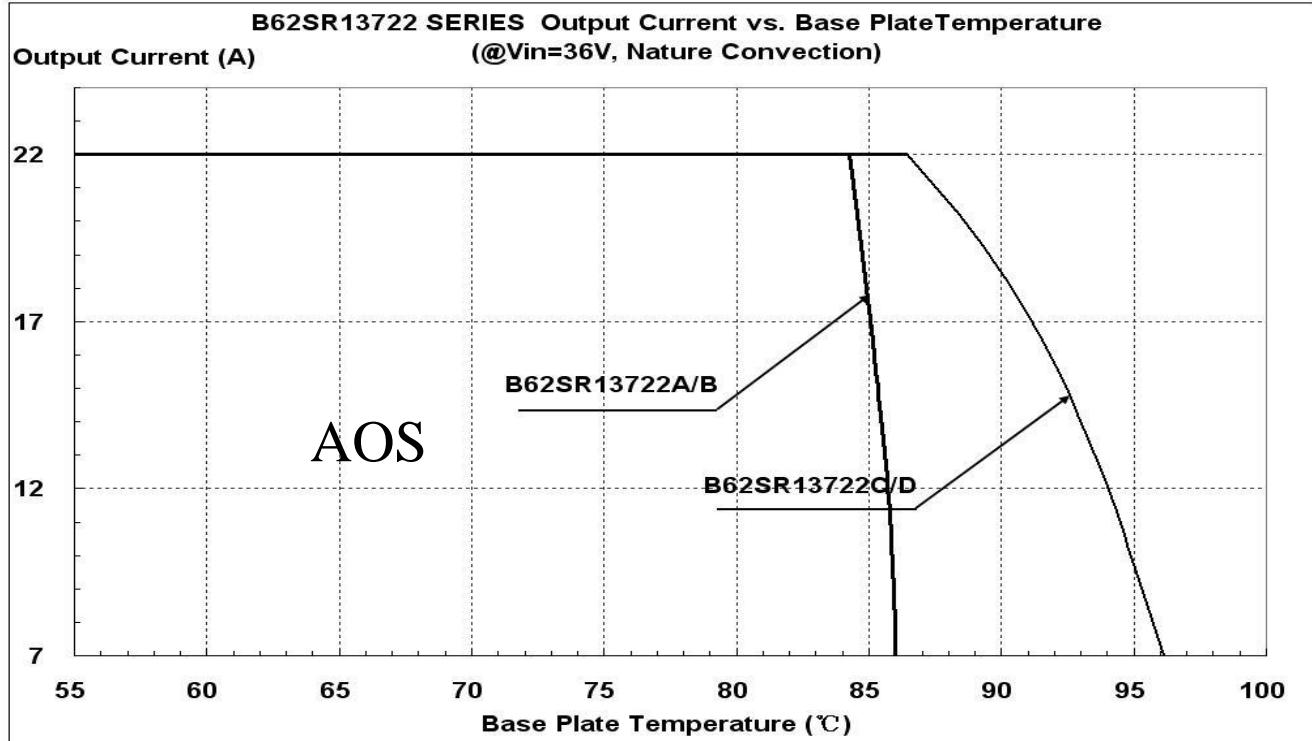
Figure 24: Output Current vs. Base Table temperature @ Vin=36V
