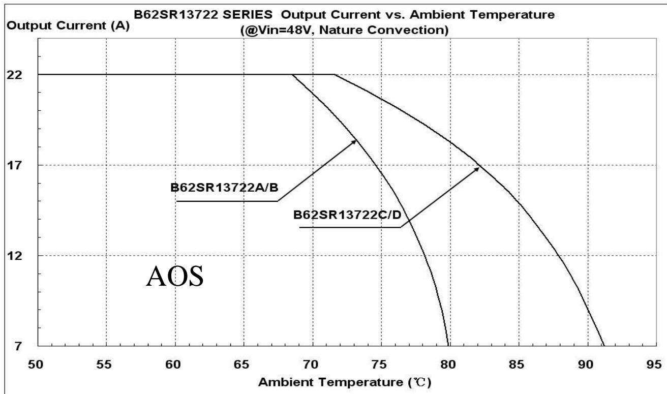
Figure 19: Output Current vs. Ambient temperature @ Vin=48V
