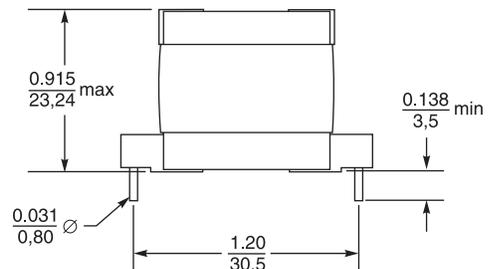
Dimensions are in  $\frac{\text{inches}}{\text{mm}}$
