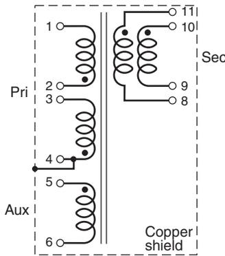
Primary windings to be connected in series and secondary windings to be connected in parallel on PC board.
