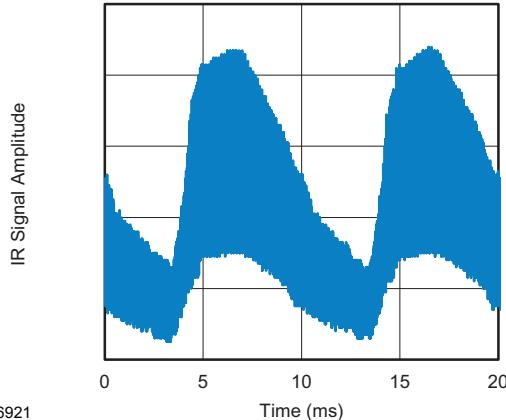
Fig. 14 - IR Disturbance from Fluorescent Lamp
