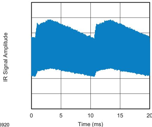
Fig. 13 - IR Disturbance from Fluorescent Lamp
