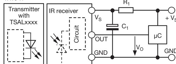
R<sub>1</sub> and C<sub>1</sub> recommended to reduce supply ripple for V<sub>S</sub> < 2.8 V
