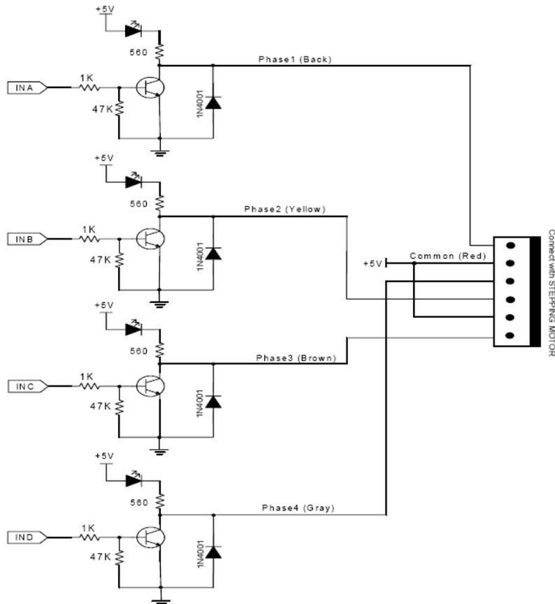
FIG 2: MR-MINI-STEP-MOTOR Schematic
