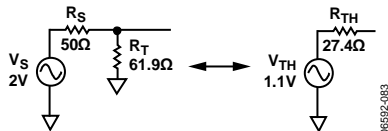
Figure 63. Calculating Thevenin Equivalent
