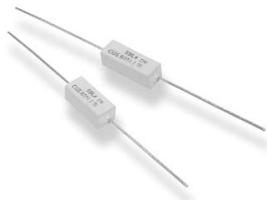
The SBL Series is a low ohmic non-inductive resistor with a low temperature coefficient in a fully insulated ceramic housing. It is ideal for applications in power supply regulation, motor control current monitoring, feedback control loops, overload sensors and radio frequency applications. The solid metal element has welded copper terminals and is encapsulated in a ceramic housing, filled with compressed silica sand.
