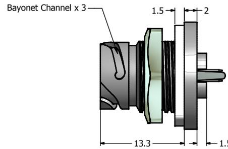
Ⓘ Sealed with Sealing Compound, provides IP67 even when uncovered (For potted version only)
