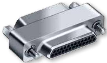
These connector savers feature a one-piece aluminum housing, TwistPin contacts and locking hardware. Typical applications include test equipment and space-grade instruments. The Micro-D Sav-Con® prevents wear and tear on sensitive gear. Standard versions are electroless nickel plated. Other plating finishes are available on request.
