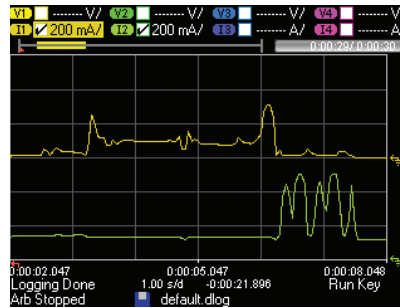
Figure 6. In Data Logger View, you can log data on multiple traces. Here, the current flowing out of output 1 and output 2 are captured over 30 seconds.
