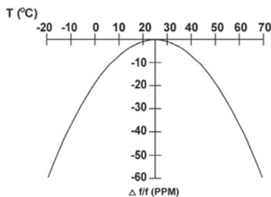
To determine frequency stability, use parabolic curvature (K).
