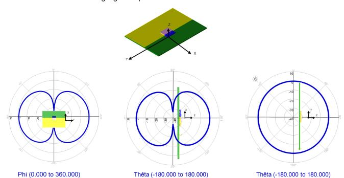
Gain measurement in dBi @ 2.45 GHz.
