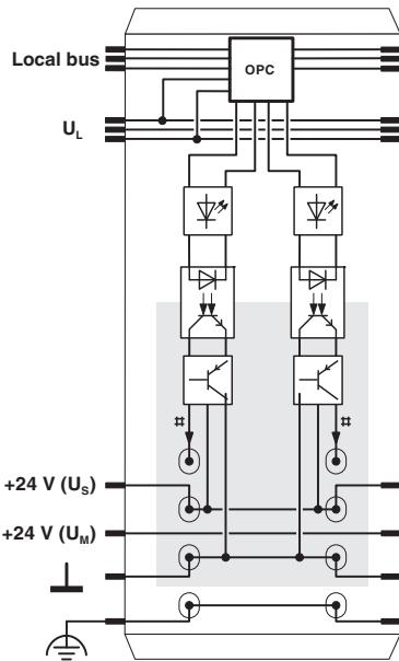
Figure 2 Internal wiring of the terminal points
