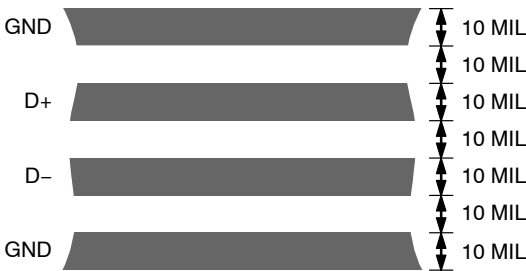
Figure 18. Typical Arrangement of Signal Tracks
