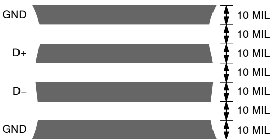
Figure 18. Typical Arrangement of Signal Tracks
