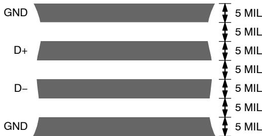
Figure 22. Typical Arrangement of Signal Tracks
