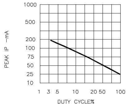
Fig.6 MAX PEAK CURRENT VS. DUTY CYCLE % (REFRESH RATE f=1KHz)
