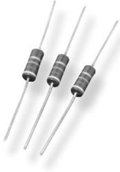
The CBT series of resistors is constructed utilising solid carbon composition, which is the traditional medium for absorbing high energy pulses, in cases of high inrush current. These resistors have evolved over many years to have excellent pulse withstand capabilities, whilst remaining very stable. These improved characteristics have been achieved by prudent selection of materials of optimum physical properties and by advances in the manufacturing process.
