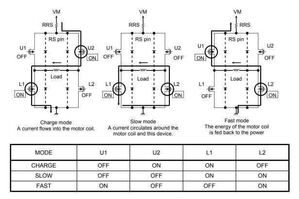
This IC controls the motor current to be constant by 3 modes listed above.
