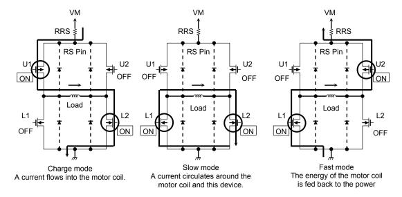
**Output transistor operational function**
