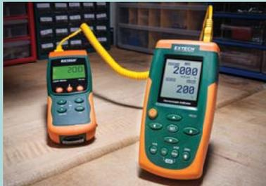
Source and measure 8 thermocouple type devices (J, K, T, E, C, R, S and N) with one meter that provides precision output displayed as °C/°F or mV.
