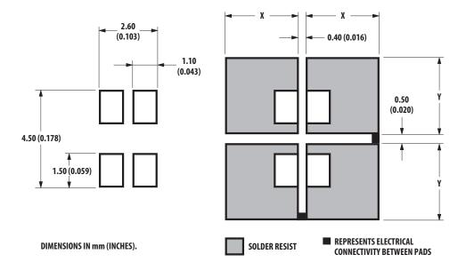
Figure 10: Recommended Soldering Pad Pattern (TTW)
