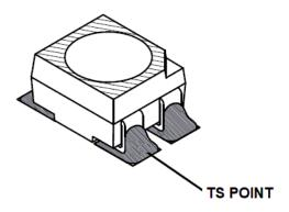
$\mathsf{T}_S$  can be measured easily by mounting a thermocouple on the soldering joint as shown in the preceding figure, while  $\mathsf{R}_{\theta\mathsf{J-S}}$  is provided in the data sheet. Verify the  $\mathsf{T}_S$  of the LED in the final product to ensure that the LEDs are operating within all maximum ratings stated in the data sheet.
