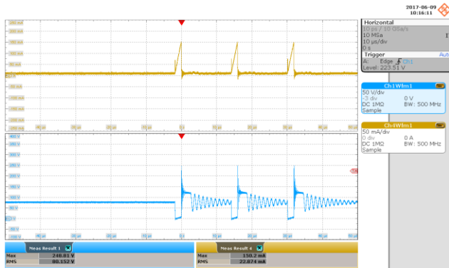
Figure 29 – 85 VAC Input. Condition: 3.8 V – 20 mA, 12 V – 0 A. Upper: I_{DRAIN} , 50 mA / div. Lower: V_{DRAIN} , 50 V / div., 10 \mu s / div.
