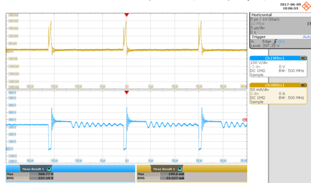
Figure 32 – 265 VAC Input. Condition: 3.8 V – 20 mA, 12 V – 20 mA. Upper: I_{DRAIN} , 50 mA / div. Lower: V_{DRAIN} , 100 V / div., 5 \mu s / div.
