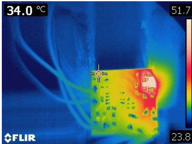
Figure 15 – Measured Temperature at 0.3 W, Ambient Temperature = 24 °C. D2 – 12 V Output Diode. Spot Temperature = 34 °C.
