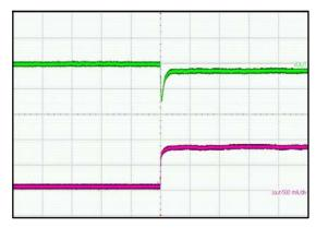
$(V_{IN}=5~V,~I_{LOAD}=100~mA,~L=2.2~\mu H,~C_{OUT}=2~x~22~\mu F)$  Upper Trace: Output Dynamic Voltage, 100 mV/div Lower Trace: Output Current, 500 mA/div
