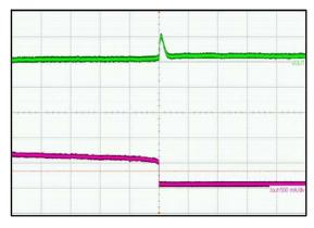
(V<sub>IN</sub> = 5 V, I<sub>LOAD</sub> = 100 mA, L = 2.2  $\mu$ H, C<sub>OUT</sub> = 2 x 22  $\mu$ F) Upper Trace: Output Dynamic Voltage, 100 mV/div Lower Trace: Output Current, 500 mA/div Time Scale: 200  $\mu$ s/div
