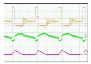
$(V_{IN}=5~V,~I_{LOAD}=120~mA,~L=2.2~\mu H,~C_{OUT}=2~x~22~\mu F)$  Upper Trace: Lx Pin Switching Waveform, 2 V/div Middle Trace: Output Ripple Voltage, 20 mV/div Lower Trace: Inductor Current, 200 mA/div
