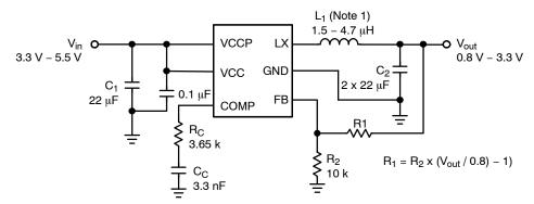
Figure 2. NCP1599 Application Circuit
