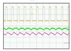
$(V_{IN}=5~V,~I_{LOAD}=1.5~A,~L=2.2~\mu H,~C_{OUT}=2~x~22~\mu F)$  Upper Trace: L<sub>X</sub> Pin Switching Waveform, 2 V/div Middle Trace: Output Ripple Voltage, 20 mV/div Lower Trace: Inductor Current, 1 A/div
