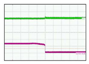
(VIN = 5 V, I<sub>LOAD</sub> = 100 mA, L = 2.2 H, C<sub>OUT</sub> = 2 x 22  $\mu$ F) Upper Trace: Output Dynamic Voltage, 100 mV/div Lower Trace: Output Current, 500 mA/div Time Scale: 200  $\mu$ s/div
