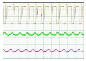
$(V_{IN}=5~V,~I_{LOAD}=120~mA,~L=2.2~\mu H,~C_{OUT}=2~x~22~\mu F)$  Upper Trace:  $L_X$  Pin Switching Waveform, 2 V/div Middle Trace: Output Ripple Voltage, 20 mV/div Lower Trace: Inductor Current, 1 A/div
