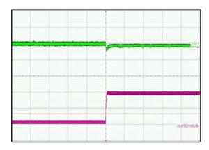
(V<sub>IN</sub> = 5 V, I<sub>LOAD</sub> = 100 mA, L = 2.2 H, C<sub>OUT</sub> = 2 x 22  $\mu$ F) Upper Trace: Output Dynamic Voltage, 100 mV/div Lower Trace: Output Current, 500 mA/div Time Scale: 200  $\mu$ s/div
