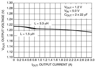
Figure 13. Load Regulation for V<sub>OUT</sub> = 1.2 V
