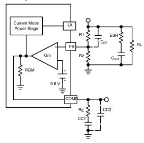
Figure 26. NCP1599 Compensation Components
