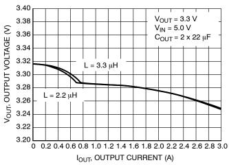
Figure 9. Load Regulation for V<sub>OUT</sub> = 3.3 V
