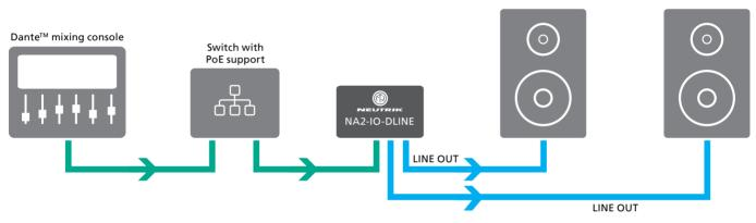
Loudspeakers and amplifiers that do not support  $Dante^{TM}$  can be connected to a  $Dante^{TM}$  network using the  $Dante^{TM}$  adapter.
