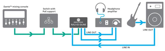
Using the Dante<sup>™</sup> adapter, the two applications described above can also be operated simultaneously (= mixed mode).
