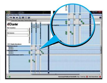
The "Dante<sup>™</sup> Controller" software is solely used to set up the audio connection (routing) between devices and to configure the involved devices.
