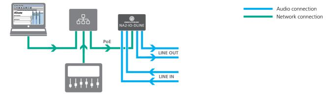
The Dante<sup>™</sup> adapter forwards information to the PoE switch indicating that it is a "Class 1" device to ensure the correct power supply.
