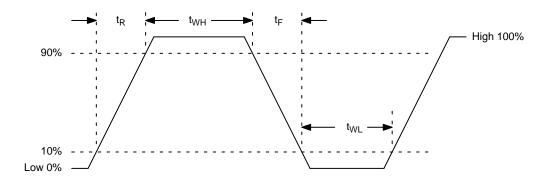
Figure 14. CCD Clock Waveform
