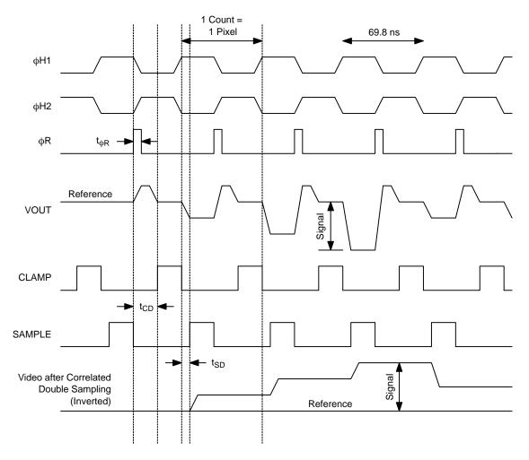
Figure 12. Pixel Timing
