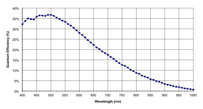
Figure 8. Monochrome with Microlens Quantum Efficiency
