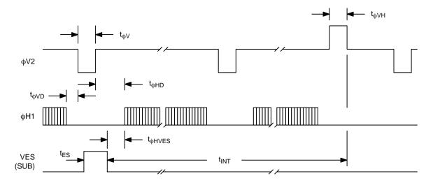
Figure 13. Electronic Shutter Timing
