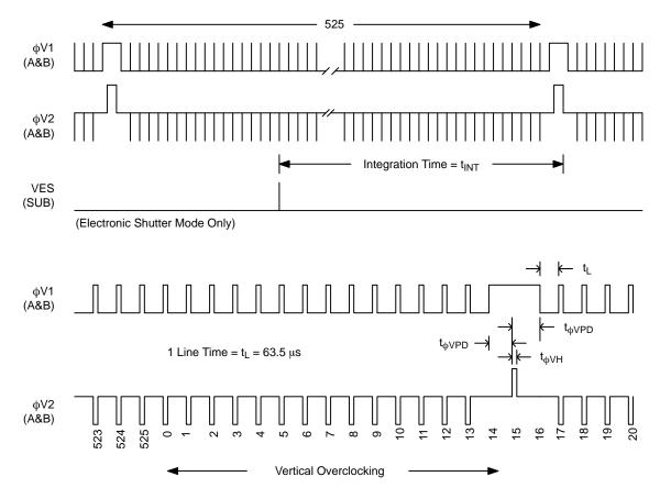
NOTE: When no electronic shutter is used, the integration time is equal to the frame time.
