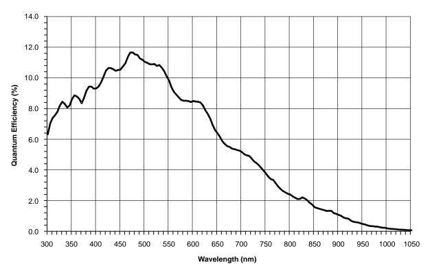
Figure 9. Monochrome, No Microlens, No Cover Glass Quantum Efficiency
