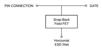
Figure 4. Internal Protection Circuit for  $\varphi H1$  and  $\varphi H2$
