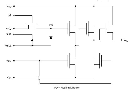
Figure 3. Output Structure
