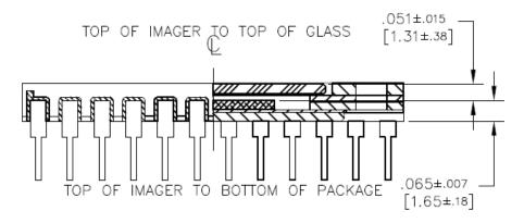
Figure 16. Die to Package Alignment
