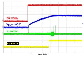
FIGURE 22. SOFT-START AT NO LOAD (PFM)
