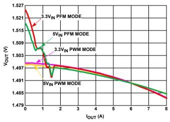
FIGURE 12.  $V_{OUT}$  REGULATION vs LOAD (1MHz,  $V_{OUT}$  = 1.5V)
