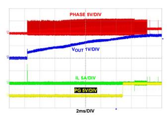
FIGURE 31. OUTPUT SHORT-CIRCUIT RECOVERY
