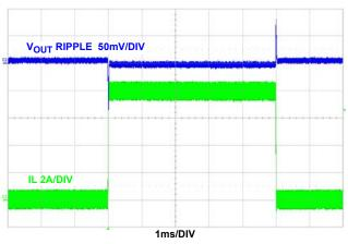
FIGURE 19. LOAD TRANSIENT (PWM)
