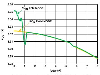
FIGURE 15.  $V_{OUT}$  REGULATION vs LOAD (1MHz,  $V_{OUT}$  = 3.3V)
