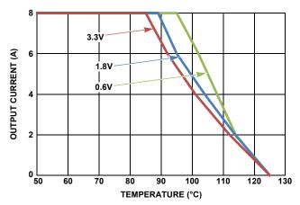
FIGURE 38. DERATING CURVE vs TEMPERATURE
