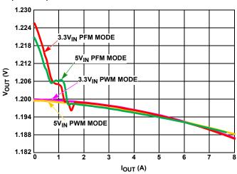
FIGURE 11. V<sub>OUT</sub> REGULATION vs LOAD (1MHz, V<sub>OUT</sub> = 1.2V)
