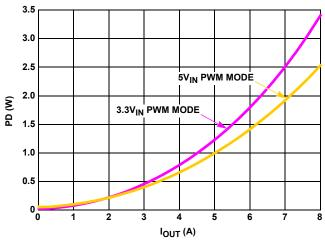
FIGURE 8. POWER DISSIPATION vs LOAD (1MHz, V<sub>OUT</sub> = 1.8V)
