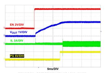
FIGURE 21. SOFT-START WITH NO LOAD (PWM)
