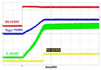
FIGURE 24. SOFT-START AT FULL LOAD
