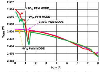
FIGURE 14.  $V_{OUT}$  REGULATION vs LOAD (1MHz,  $V_{OUT} = 2.5V$ )
