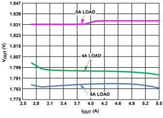
FIGURE 10.  $V_{OUT}$  REGULATION vs  $V_{IN}$  (PFM  $V_{OUT} = 1.8V$ )
