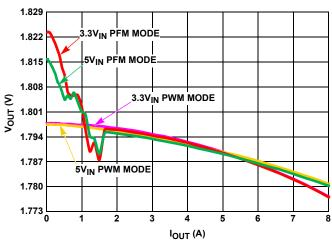
FIGURE 13.  $V_{OUT}$  REGULATION vs LOAD (1MHz,  $V_{OUT}$  = 1.8V)
