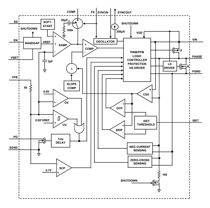
FIGURE 3. FUNCTIONAL BLOCK DIAGRAM
