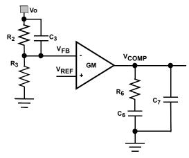
FIGURE 41. TYPE II COMPENSATOR
