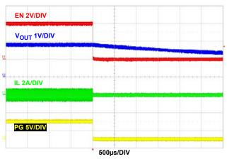
FIGURE 25. SOFT-DISCHARGE SHUTDOWN
