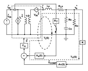
FIGURE 40. SMALL SIGNAL MODEL OF SYNCHRONOUS BUCK REGULATOR
