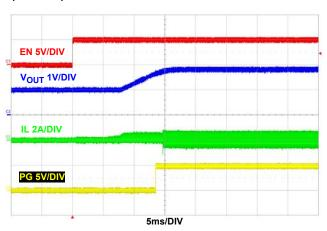
FIGURE 23. SOFT-START WITH PREBIASED 1V
