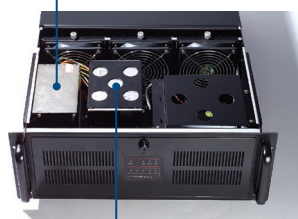
Extra drive bay which can hold up to three 3.5" HDDs
